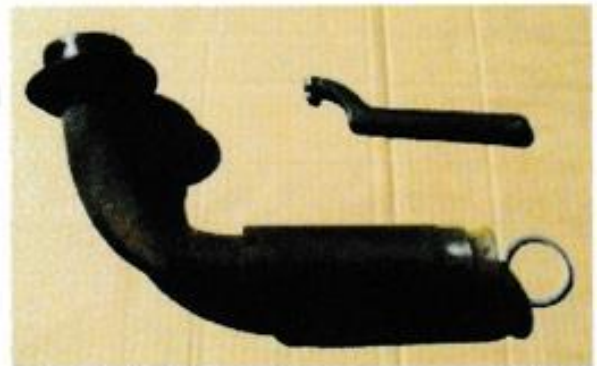
Filler tube, lead seal on right, spanner wrench above
